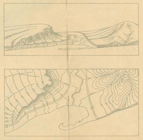
The sketch represents a river valley that lies between two hills. In the foreground is the sea, with a bay that is partly inclosed by a hooked sand bay. On each side of the valley is a terrace into which small streams have cut narrow gullies. The hill on the right has a rounded summit and gently sloping spurs separated by ravines. The spurs are truncated at their lower ends by a sea cliff. The hill at the left terminates abruptly at the valley in a steep scarp, from which it slopes
